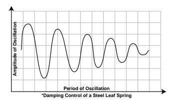
The Equalizer has the same initial amplitude, but see the swift dampening with quick return to stability.
