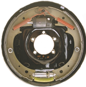
Uniservo right hand brake shown
